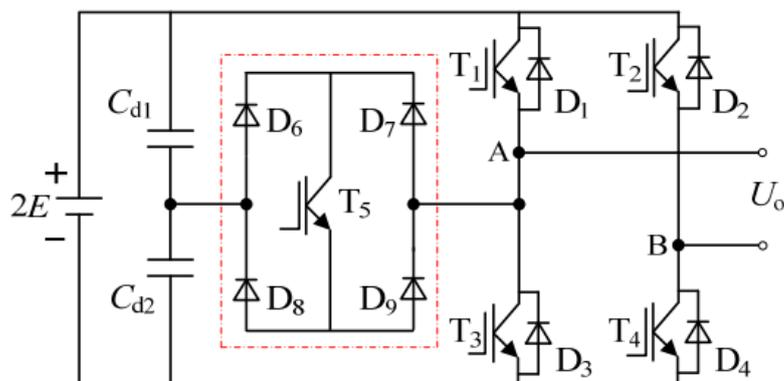
Fig. 1. Circuit diagram of a T-type five-level inverter.
