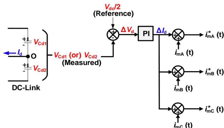
Fig. 4. Block-diagram of the DC-link Capacitor Voltage Control.
