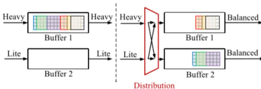
Fig 2: Adaptive distribution aimed at workload equilibrium (a) deprived of adaptive distribution and (b) through adaptive spreading.
