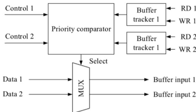
Fig 6: Circuit building for projected adaptive load distribution.
