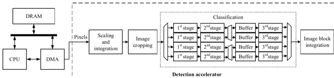
Fig 1: Complete construction of the planned traffic symbol detection system.
