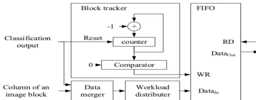
Fig 5: Circuit construction for projected collective image storage
