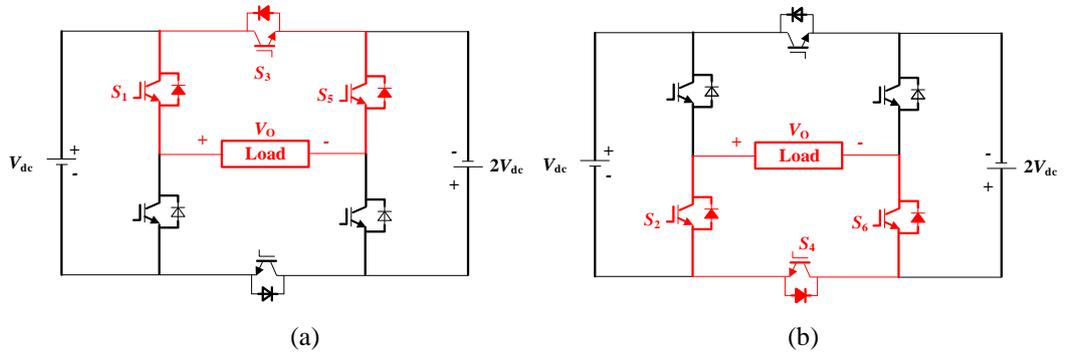
Fig. 2. Operating states: (a) Positive Zero-crossing (b) Negative Zero-crossing.
