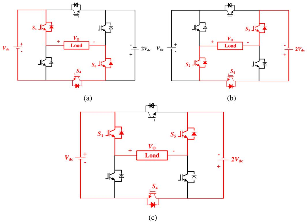
Fig. 3. Positive-level operating states: (a)  $V_O = V_{dc}$ , (b)  $V_O = 2V_{dc}$  and (c)  $V_O = 3V_{dc}$ .
