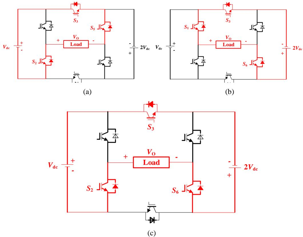
Fig. 4. Negative-level operating states: (a)  $V_0 = -V_{dc}$ , (b)  $V_0 = -2V_{dc}$  and (c)  $V_0 = -3V_{dc}$ .
