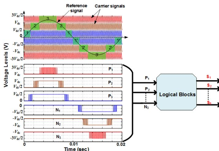
Fig. 5. Sine-triangle comparison PWM scheme.
