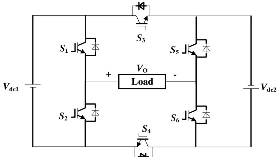
Fig. 1. Circuit diagram of the proposed configuration.
